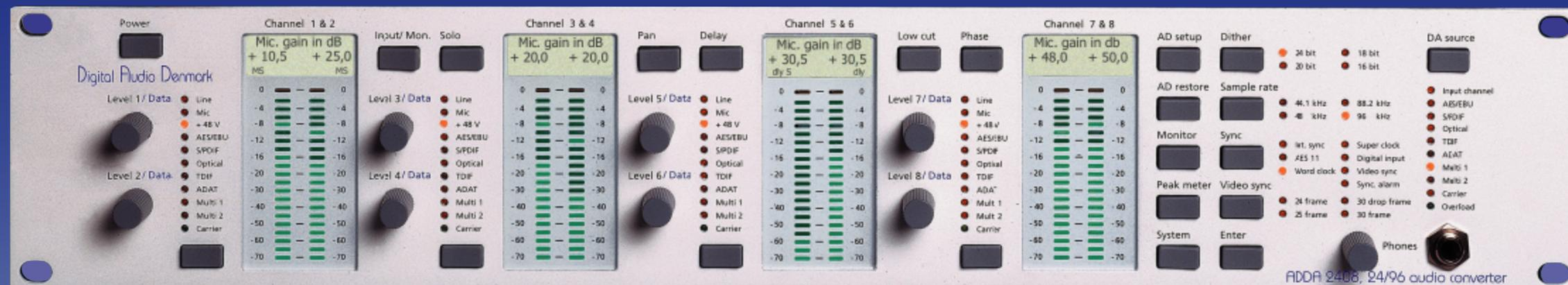
**Supreme microphone preamplifier** with low cut filter and phase inverse selection. The preamplifier has an equivalent input noise of 131 dB. The level control can set the gain in 0,5 dB steps from 0 to + 99 dB for precise control of the analog input level. This enable the user to scale the microphone level optimally into the 117dB dynamic range provided by the A/D converter.
